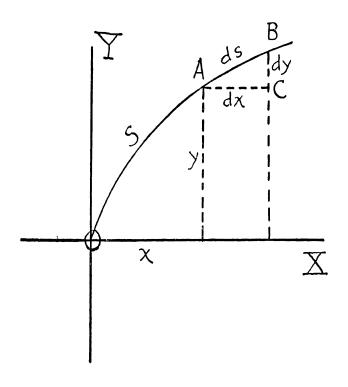
is no longer the hypotenuse of a right triangle, and of course we CANNOT write here  $s^2 = x^2 + y^2$ !
