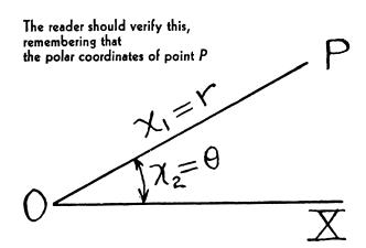
(1) its distance,  $x_1$ , from a fixed point, O, (2) the angle,  $x_2$ , which OP makes with a fixed line OX. Then (8) is obvious from the following figure:
