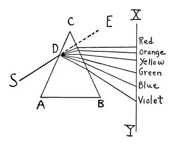
When a beam of white light, SD, strikes the prism ABC, it does NOT continue in the SAME direction, DE, but is bent.\*
