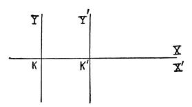
And x in this case is the distance from K to K', that is, the distance traversed, in time t by K' moving with velocity v relatively to K.
