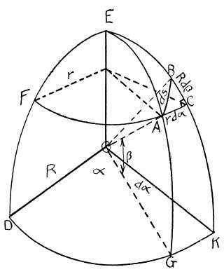
Let DE be the meridian from which longitude is measured — the Greenwich meridian. And let DK be a part of the equator, and E the north pole. Then the longitude and latitude of A are, respectively, the number of degrees in the arcs AF and AG, (or in the corresponding central angles,  $\alpha$  and  $\beta$ ). Similarly,
