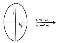
Applying this idea to the Michelson-Morley experiment, the distance AB (= a) on p. 8, becomes  $a/\beta$ , and  $t_1$  becomes  $2a\beta/c$ , instead of  $2a\beta^2/c$ , so that now  $t_1 = t_2$ , just as the experiment requires.
