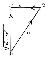
Consequently, the time required for the journey from A to C would be  $a/\sqrt{c^2-v^2}$ , where a is the distance from A to C. Similarly, in going back from C to A, it is easy to see that,
