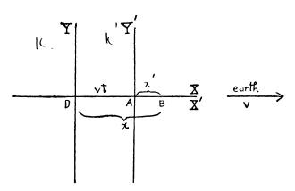
Consider a set of axes, X and Y, supposed to be fixed in the stationary ether, and another set X' and Y', attached to the earth and moving with it,
