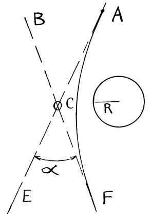
the path of a ray of light, AOE, from a star, A, when the sun is NOT in that part of the sky. And, also, when the sun IS present, and the ray is deflected and becomes ACF,
