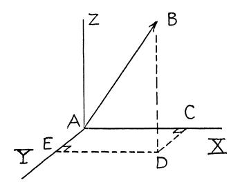
By dropping the perpendicular BD from B to the XY-plane, and then drawing the perpendiculars DC and DE to the X and Y axes, respectively, we have the three components of AB, namely, AC, AE and DB; and, as before, the components depend upon the particular choice of axes.
