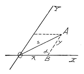
The coordinates of the point A are now represented by x and y which are measured parallel to the X and Y axes, and are now NOT at right angles to each other.
