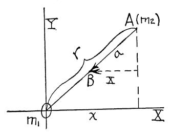
then OA = r; and let AB represent the acceleration at A(since  $m_2$  is being pulled toward  $m_1$ ) in both magnitude and direction. Now if X is the x-component of a, it is obvious that
